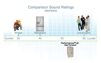
Carrier manufactures gas furnaces that are among the quietest in the industry. We test our products in a sound laboratory specifically built to resemble a typical residence. Sound level recordings produced at steady state, single-stage operation (the most common operating condition), measured three feet from furnace. Other sound levels, mentioned for comparison, as published at http://www.noisyplanet.nidcd.nih.gov/SiteCollectionDocuments/Bookmark\_2up.pdf.
