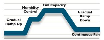
Gradual ramp up and down of the variable-speed motor significantly reduce sound
